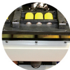
采用橡胶轮压紧 Clamp is rubber roller
