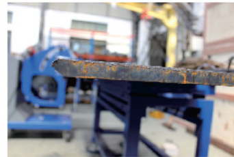
加工小板 Process "X" of bevel type
