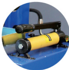
液压调高 Hydraulic height adjustment
