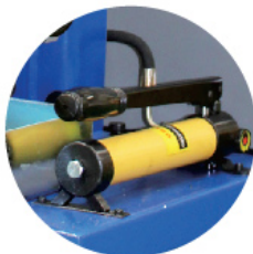
液压调高 Hydraulic height adjustment
